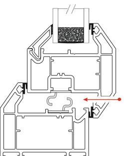
**STAY GUARD ELITE SG036** on outer frame and sash for all types of stays to include Egress/Easy Clean
